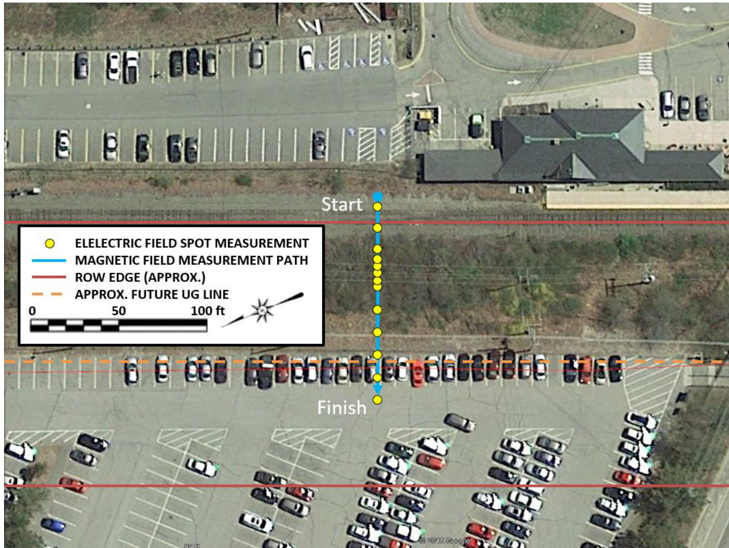
Figure C-2. Aerial photograph of measurement Site 2 (UNH Parking Lot A) showing the approximate location of the magnetic-field measurement path and electric-field spot measurements performed on June 6, 2019.
